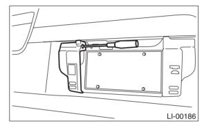
3) Remove cover. Turn the socket and remove the bulb.
