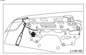
2) Back off license plate bracket and remove bolts.
