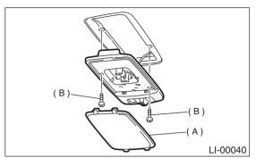
3) Disconnect harness connectors and remove the light.
