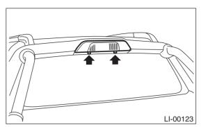
2) Turn the socket and remove the bulb.
