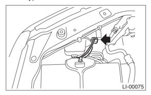
4) Remove three bolts and disconnect connectors, and then detach headlight assembly.
