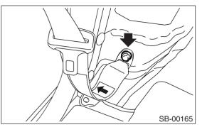
3) Remove webbing guide bolts, and then detach outer belt side.
