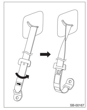
3) Install lower anchor bolt.
