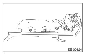
23) Remove 2 bolts, and then remove slide rail.
