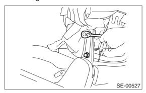
7) Remove hinge screw cover and screws, and remove seat back from hinge.
