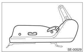
21) Remove the cover on the underside of the seat hinge, remove the two bolts, and remove the seat hinge.
