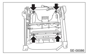
14) Remove hook clips on back side of seat cushion, and remove wire rings.
