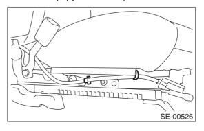
6) Turn cover and cushion, and remove the two bolts from hinge.
