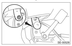
8) While picking up tip with a plier, remove head-rest lock bushing.
