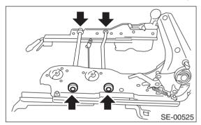
25) Remove 2 bolts, and then remove slide rail.
