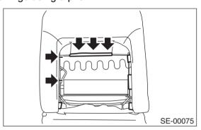
5) Remove clamp of seat heater wire harness. (Seat heater equipped vehicle)
