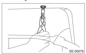
9) Remove hog ring (A) on front face of seat.
