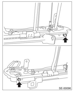
24) Remove 4 screws, and then remove hinge.
