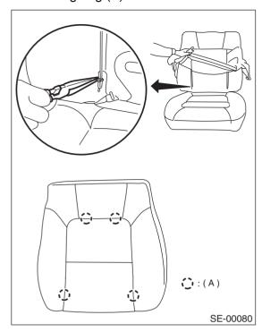
10) Remove hog rings, and then remove seat heater. (Seat heater equipped vehicle)
