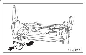
20) Remove the reclining lever cover and screw, disconnect the seat switch connector on the underside of the cover, and remove the hinge cover.
