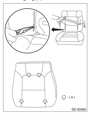
10) Remove wire rings, and then remove seat heater. (Seat heater equipped vehicle)
