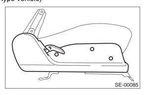
14) Remove the 4 bolts of seat hinge assembly, and then remove seat cushion.
