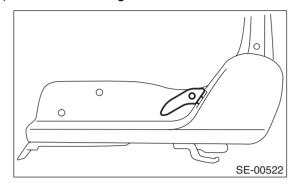
21) Remove hinge cover cap and screws.
