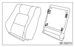
4) Remove hook on back side of seat, and remove wire rings using a plier.
