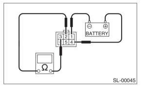
If the measured value is out of specifications indicated in table, replace security horn relay. If NG, replace door lock actuator.
