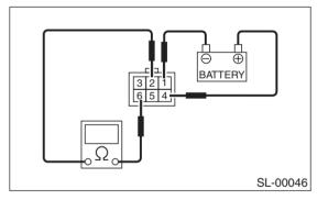
If the measured value is out of specifications indicated in table, replace security horn relay.
