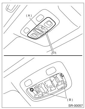
3) Disconnect harness connectors and remove sunroof switch.
