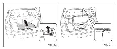
To open the lid, pull the handle up. To keep the lid open, hang the hook provided on the backside of the lid on the rear edge of the roof. The spare tire is stored under the storage tray.
