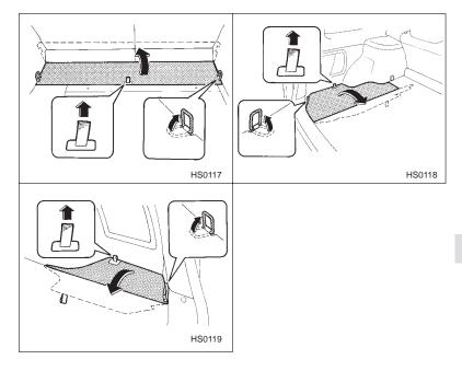
To open the lid, raise the cargo anchorage eyelets and pull the tab up. The jack and jack handle are stored in the left side storage tray.
