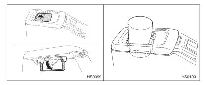
The front passenger's cup holder is built in the lid of the center console. To use the cup holder, open the lid by sliding it forward and unfold the arm. Adjust the opening area by sliding the lid forward or rearward to fit the cup. When not in use, fold the arm and close the lid.
