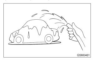
CHECK : Does water leak into the passenger compartment when showering vehicle?
