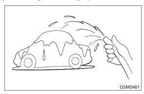
CHECK : Does water leak into the passenger compartment when showering vehicle?
