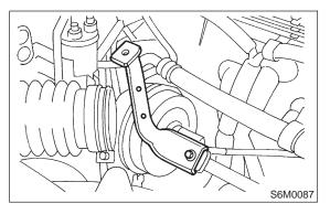
4) Remove cruise control cable end from throttle cam.
