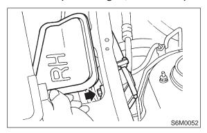
5) Remove bolts which secure sleeve unit.
