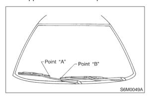
3) Adjust washer ejecting point on windshield glass as shown in figure when vehicle stops.
