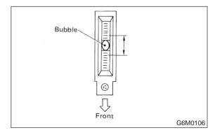
3) Look at the beam angle gauge (horizontal movement). The center mark (the red line on the inner scale) should not deviate from the red line on the outer case.
