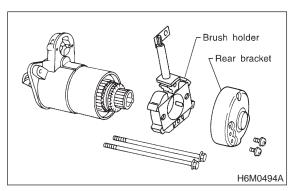
4) Remove armature and yoke. Ball used as a bearing will then be removed from the end of armature.
