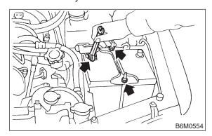
3) Remove washer tank mounting bolts.
