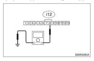
(CHECK): Is the resistance less than 10  $\Omega$ ?
