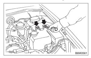
4) Disconnect washer tank connectors.
