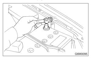
2) Disconnect connector and terminal from generator.
