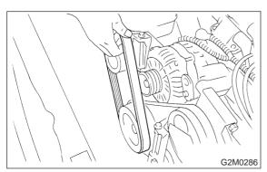
5) Remove bolts which install generator onto bracket.
