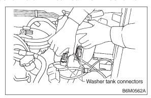
5) Move washer tank upward.
