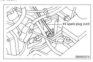
7) For subsequent procedures, refer to the procedure for #1 spark plug. <Ref. to 6-1 [W3A1].>
