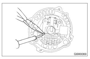
5) Remove the brushes by unsoldering at the pigtails.
