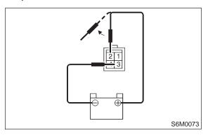
3) Reconnect battery and ensure that wiper motor stops at "AUTO STOP" after it has been operated.
