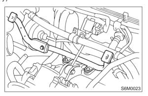
4) Disconnect connector and terminal from starter.
