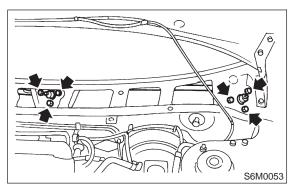
6) Remove wiper link from service hole in front panel.
