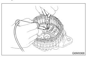
4) Remove screws which secure IC regulator to rear cover, and unsolder connection between IC regulator and rectifier to remove IC regulator.
