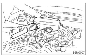
3) Disconnect connector from ignitor.
