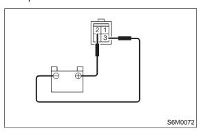
2) Check wiper motor for proper stoppage: After operating wiper motor, disconnect battery from wiper motor.
