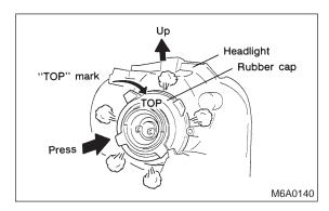
• To keep water out, correctly engage the groove portion of the rubber cap.
