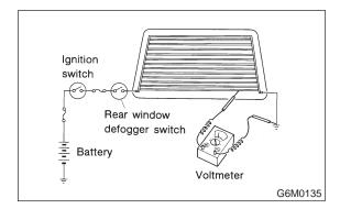
• When measuring voltage, wind a piece of tin foil around the tip of the tester probe and press the foil against the wire with your finger.
