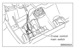
4) Remove main switch by pushing it outward.
