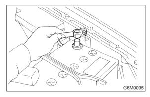
2) Disconnect mass air flow sensor connector.
