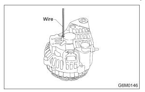
2) Heat the rear bracket [50 to 60°C (122 to 140°F)] and press the rear bearing into the rear bracket. Then lubricate the rear bracket.
