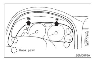
3) Remove screws which secure combination meter, and pull combination meter out.
