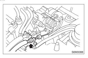
5) Disconnect cruise control vacuum hose from intake manifold.
