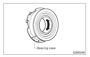
3) Check wear and damage of bearing case surface contacting with lever.
