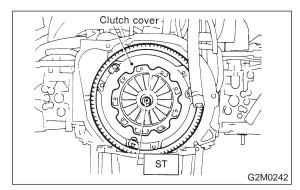
2) Remove clutch cover and clutch disc.
