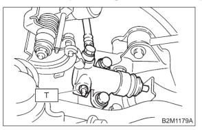
6) After depressing the clutch pedal, make sure that there are no leaks evident in the entire system.7) After bleeding air from system, ensure that clutch operates properly.
