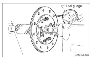
5) Worn spline, loose rivets and torsion spring failure
