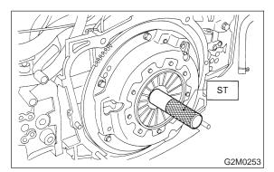
4) Install clutch cover on flywheel and tighten bolts to the specified torque.
