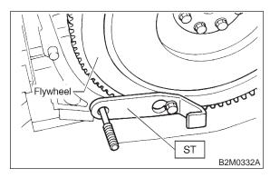
2) Tighten the flywheel attaching bolts to the specified torque.
