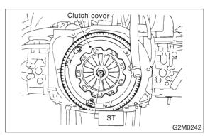
2) Remove clutch cover and clutch disc.
