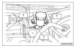
2) Connect push rod of master cylinder to clutch pedal, and install clevis pin and snap pin.
