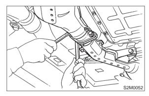
7) Remove bolts which hold front exhaust pipe onto cylinder heads.
