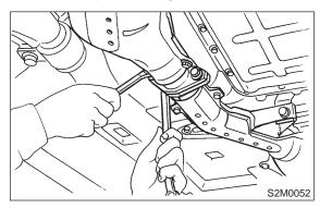
4) Connect rear oxygen sensor connector. (Except California spec. vehicles)
