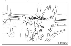
4) Separate center exhaust pipe and rear catalytic converter assembly from rear exhaust pipe.
