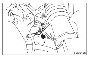
7) Connect front oxygen sensor connector.
