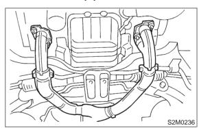
1. Front Catalytic Converter
