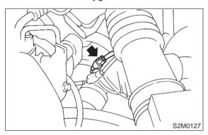
3) Disconnect rear oxygen sensor connector. (California spec. vehicles)
