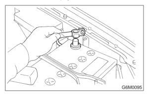
2) Disconnect front oxygen sensor connector.
