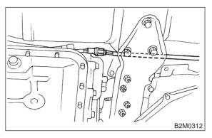
6) Separate center exhaust pipe from front catalytic converter.
