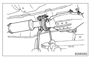
4) Tighten bolt which holds center exhaust pipe to hanger bracket.
