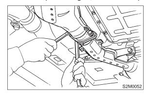
3) Install center exhaust pipe to rear exhaust pipe.
