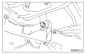
5) Connect rear oxygen sensor connector. (Except California spec. vehicles)
