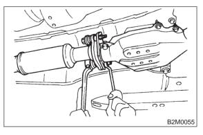
5) Separate center exhaust pipe and rear catalytic converter assembly from front catalytic converter.
