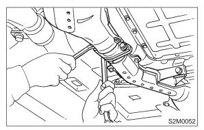
6) Remove center exhaust pipe and rear catalytic converter assembly from hanger bracket.
