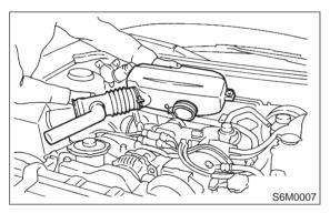
3) Remove bolt which installs purge control solenoid valve to intake manifold.
