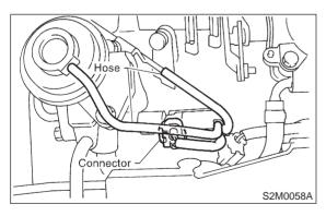
5) Remove bolt which installs EGR solenoid valve onto intake manifold.
