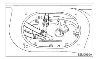
6) Remove nuts which install fuel pump assembly onto fuel tank.
