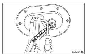
10) Remove bolt which installs fuel level sensor on mounting bracket.
