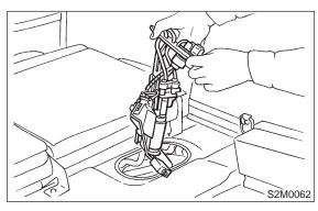
8) Disconnect connector from fuel pump bracket.
