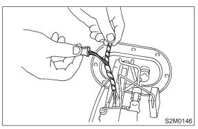
10) Remove No. 2 and No. 3 terminals from sensor connector.
