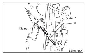
12) Remove screw which installs fuel level sensor on mounting bracket.
