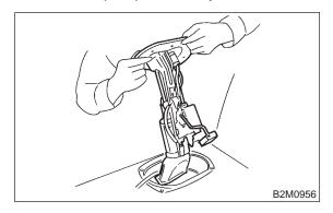
9) Disconnect connector from fuel pump bracket.
