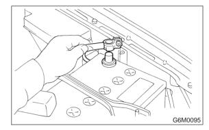
4) Disconnect quick connector, and disconnect fuel delivery hose (A). <Ref. to 2-8 [W6A0].>
