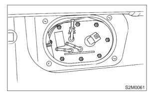
7) Take off fuel pump assembly from fuel tank.
