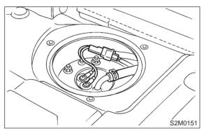
4) Remove bolts which install sub fuel level sensor on fuel tank.
