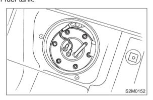
5) Remove sub fuel level sensor.
