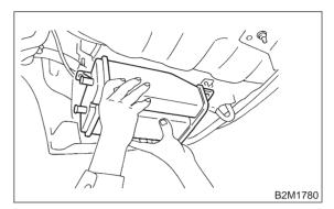
4) Disconnect connector from drain valve.
