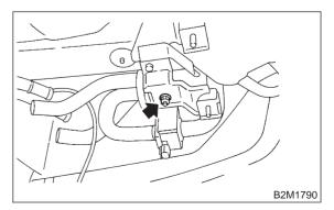
7) Disconnect evaporation hoses, and remove air filter.
