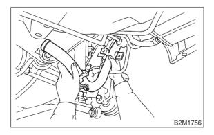
6) Disconnect evaporation hoses from shut valve.
