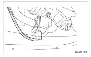
5) Disconnect evaporation hoses from drain valve.
