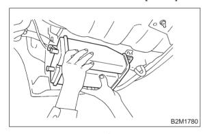
4) Disconnect connector from drain valve.
