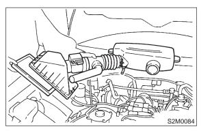
(3) Connect connector to mass air flow sensor.
