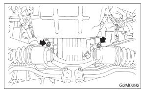
9) Tighten nuts which install front cushion rubber onto crossmember.
