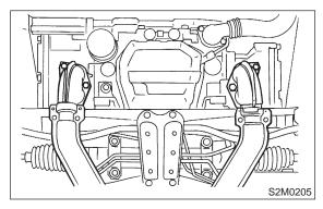
(3) Disconnect connector from rear oxygen sensor. (Except California spec. vehicle)
