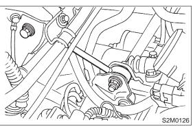
18) Disconnect fuel delivery hose, return hose and evaporation hose.
