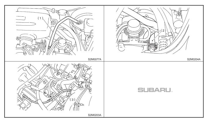
12) Remove power steering pump from bracket.(1) Loosen lock bolt and slider bolt, and remove front side V-belt.
