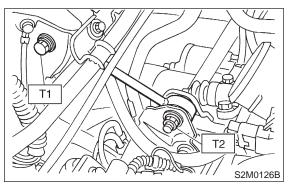
6) Install torque converter onto drive plate. (AT vehicles)
