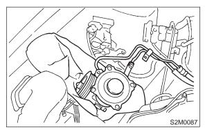
13) Remove front exhaust pipe and center exhaust pipe.
