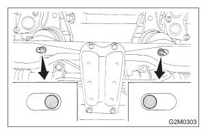
10) Install front exhaust pipe and center exhaust pipe. <Ref. to 2-9 [W1B0], [W2B0].>
