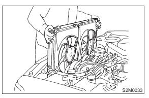
(3) Install radiator brackets and tighten bolts.
