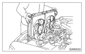
8) Collect refrigerant, and remove flexible hoses. (With A/C)
