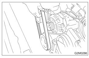
(2) Remove power steering pump bracket.
