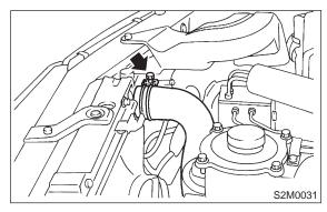
(8) Remove radiator upper bracket, and remove radiator assembly from vehicle.
