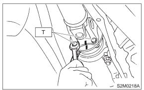
(3) Install center bearing bracket on body.
