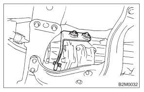
14) Drain ATF to remove ATF drain plug. (AT vehicles)
