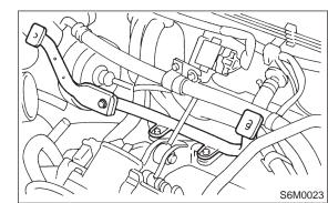
22) Install air intake duct and chamber.
