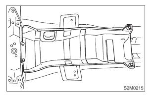
(9) Remove hanger bracket from right side of transmission.
