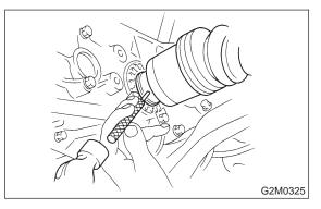
21) Remove nuts which hold lower side of transmission to engine.
