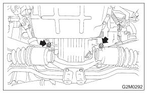
6) Tighten bolt which holds right upper side of transmission to engine.
