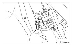
(3) Remove bolts which hold center bearing onto body.
