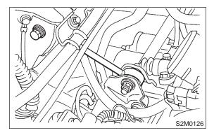
8) Separate torque converter from drive plate. (AT vehicles)
