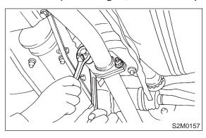
(3) Install hanger bracket on right side of transmission.
