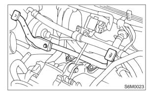
5) Disconnect the following connectors.(1) Front oxygen sensor connector
