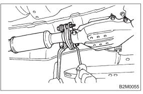
(5) Remove bolt which installs center exhaust pipe to hanger bracket.
