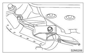
(7) Connect connector to rear oxygen sensor. (Except California spec. vehicle)
