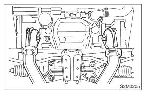
(5) Install center exhaust pipe to rear exhaust pipe.
