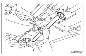
(8) Remove heat shield cover of rear exhaust pipe.
