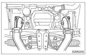
(3) Disconnect connector from rear oxygen sensor. (Except California spec. vehicle)
