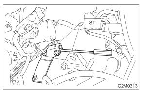
12) Remove bolt which holds right upper side of transmission to engine.
