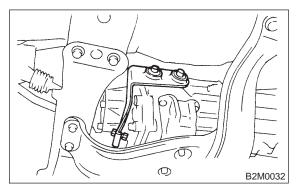
(4) Install front exhaust pipe onto engine.
