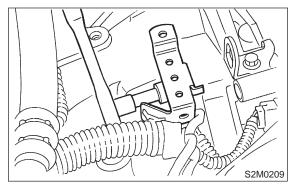
7) Install torque converter to drive plate. (AT vehicles)
