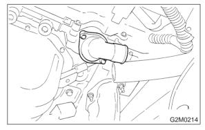
7) Install the thermostat in the intake manifold, and install the thermostat cover together with a gasket.
