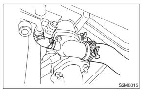
6) Remove thermostat cover and gasket, and pull out the thermostat.
