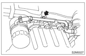
5) Disconnect radiator outlet hose and water bypass hose B (AT vehicles) from thermostat cover.
