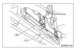
6) Disconnect radiator outlet hose and water bypass hose B (AT vehicles) from thermostat cover.
