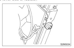
2) Install radiator while fitting radiator pins to cushions.
