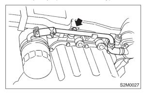
6) Remove water pipe and hoses between oil cooler and water pump. (AT vehicles only)
