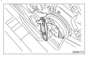
13) Remove crankshaft pulley by using ST. ST 49997700 CRANKSHAFT PULLEY WRENCH
