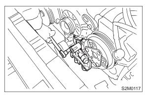
18) Remove oil pump by using flat bladed screwdriver.
