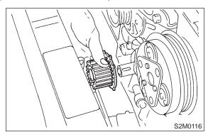
17) Remove bolts which install oil pump onto cylinder block.
