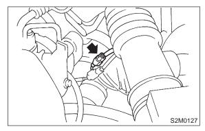
5) Disconnect rear oxygen sensor connector. (California spec. vehicles)
