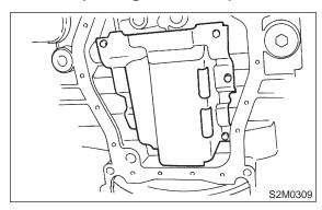
2) Install oil strainer onto baffle plate.
