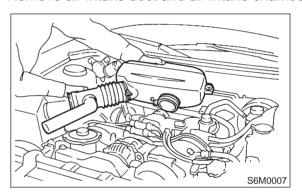
4) Disconnect front oxygen sensor connector.
