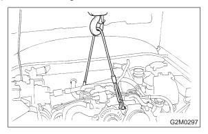
12) Connect connector to front oxygen sensor.
