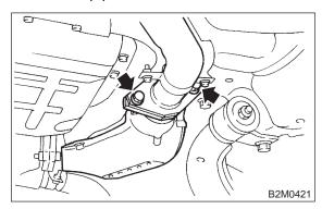
(2) Remove front exhaust pipe from engine.
