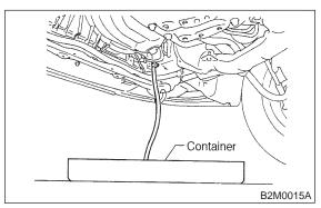
4) Remove bolt which installs water pipe to engine.
