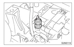
3) Connect terminal of oil pressure switch.
