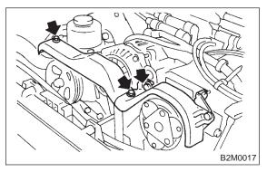
7) Connect connector and terminal to generator.
