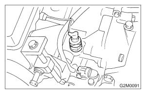
3) Remove oil pressure switch.
