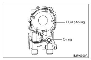
9) Install water pump and gasket.
