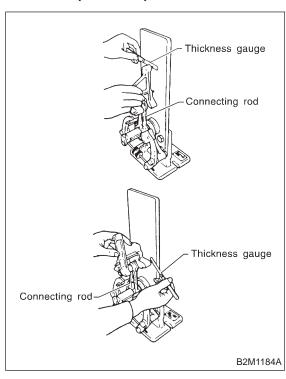
3) Install connecting rod fitted with bearing to crankshaft and measure the side clearance (thrust clearance). Replace connecting rod if the side clearance exceeds the specified limit.
