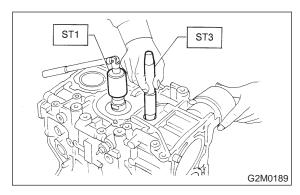
(2) Apply a coat of engine oil to piston pin and insert piston pin into piston and connecting rod through service hole.
