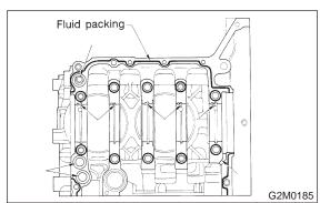
4) Temporarily tighten 10 mm cylinder block connecting bolts in alphabetical sequence shown in figure.
