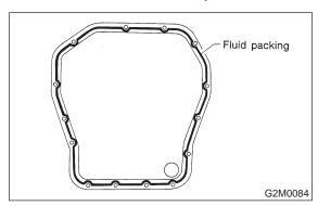
5) Apply fluid packing to matching surfaces and install oil separator cover.
