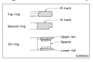
2) Squarely place piston ring and oil ring in cylinder, and measure the piston ring gap with a thickness gauge.
