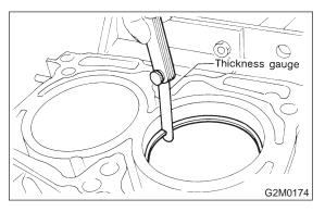
3) Measure the clearance between piston ring and piston ring groove with a thickness gauge.
