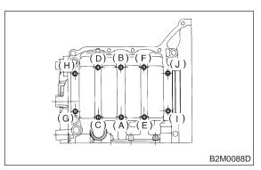
5) Tighten 10 mm cylinder block connecting bolts in alphabetical sequence.
