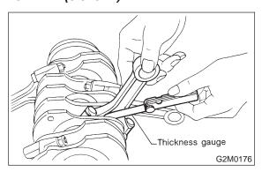
4) Inspect connecting rod bearing for scar, peeling, seizure, melting, wear, etc.
