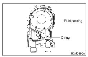
(3) Install oil pump on cylinder block. Be careful not to damage oil seal during installation.
