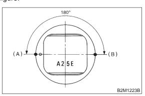
(3) Position the second ring gap at 180° on the reverse side for the top ring gap.
