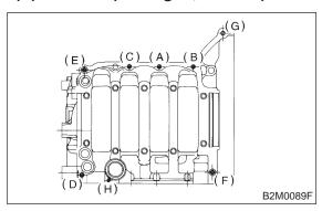
7) Install rear oil seal by using ST1 and ST2. ST1 499597100 OIL SEAL GUIDE ST2 499587200 OIL SEAL INSTALLER
