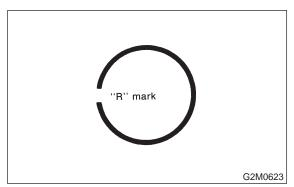
• The oil ring is a combined ring consisting of two rails and a spacer in between. When installing, be careful to assemble correctly.
