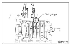
3) Inspect the crank journal and crank pin for wear. If not to specifications, replace bearing with an undersize one, and replace or recondition crankshaft as necessary. When grinding crank journal or crank pin, finish them to the specified dimensions according to the undersize bearing to be used.
