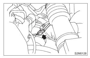
7) Connect front oxygen sensor connector.
