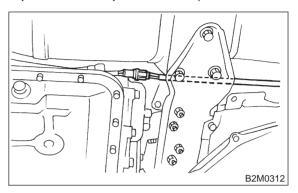
6) Separate center exhaust pipe from front exhaust pipe.
