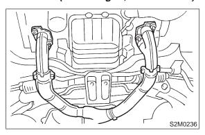
3) Install center exhaust pipe to front exhaust pipe.
