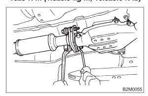
5) Tighten bolt which holds center exhaust pipe to hanger bracket.
