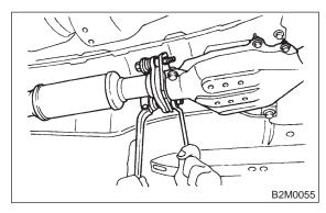
2) Separate rear exhaust pipe from muffler.
