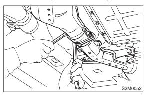
6) Remove center exhaust pipe and rear catalytic converter assembly from hanger bracket.
