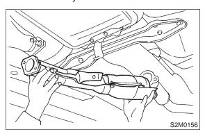
2) Temporarily tighten bolt which installs center exhaust pipe to hanger bracket.
