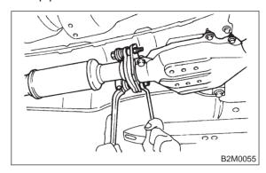
2) Separate rear exhaust pipe from muffler.
