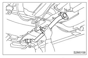
2) Install rear exhaust pipe to muffler.
