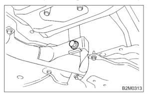
6) Connect rear oxygen sensor connector. (Except California spec. vehicles)
