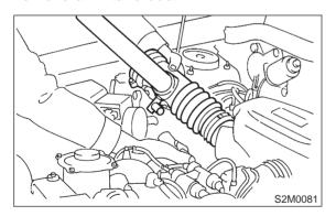
5) Disconnect connector from mass air flow sensor.
