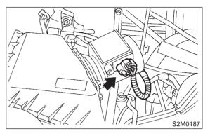
6) Remove two clips, then remove air cleaner upper cover.
