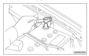
2) Loosen clamps which connect air intake duct to air intake chamber and mass air flow sensor.
