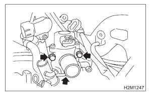
5) Install engine harness onto intake manifold.
