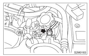
25) Disconnect connector from crankshaft position sensor.
