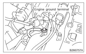
2) Disconnect connectors from throttle position sensor, ignition coil, fuel injectors, idle air control solenoid valve, purge control solenoid valve and EGR solenoid valve.
