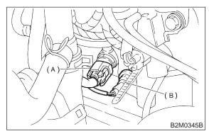
8) Install engine harness bracket, and connect engine harness connectors to bulkhead connectors.
