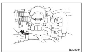
17) Disconnect engine coolant hose (A) from idle air control solenoid valve.
