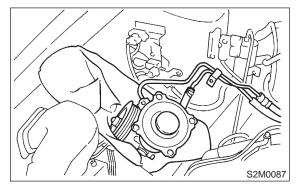
13) Disconnect spark plug cords from ignition coil.
