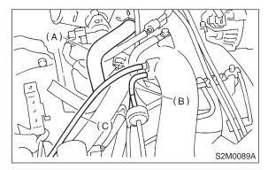
16) Connect spark plug cords to ignition coil.
