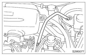
11) Connect engine coolant hose (A) to idle air control solenoid valve.
