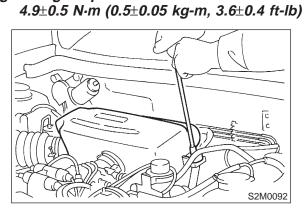
23) Connect connector to mass air flow sensor.
