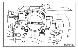
4) Install idle air control solenoid valve to intake manifold.
