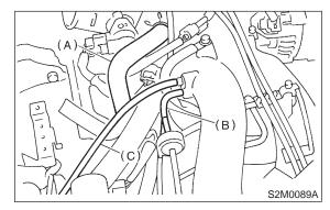
16) Disconnect engine coolant hose from throttle body.
