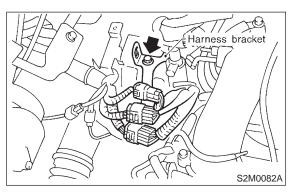
22) Disconnect connectors from engine coolant temperature sensor (A) and thermometer (B).
