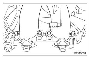
29) Remove intake manifold.
