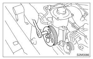
(2) Install power steering pipe brackets on right side intake manifold.
