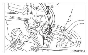
3) Connect connector to oil pressure switch.
