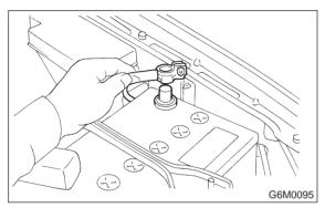
3) Disconnect connector from mass air flow sensor.
