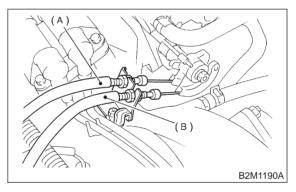
12) Remove power steering pump from bracket.(1) Remove V-belt covers.
