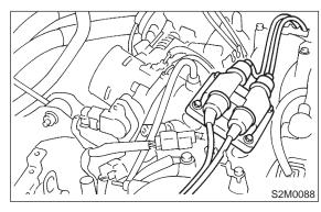
17) Install power steering pump on bracket.(1) Install power steering pump on bracket, and tighten bolts.
