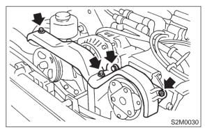
(2) Loosen lock bolt and slider bolt, and remove power steering pump drive V-belt.
