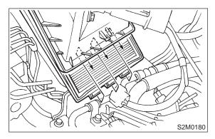
22) Tighten bolts which install air intake chamber to stays.
