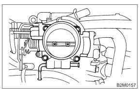
6) Remove fuel pipes, etc. from intake manifold.
