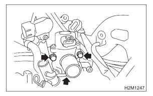
5) Remove throttle body from intake manifold.
