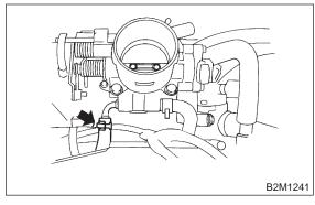
14) Connect vacuum hose (C) to cruise control diaphragm. (With cruise control models)15) Connect PCV hose (A) and vacuum hose (B) to intake manifold.
