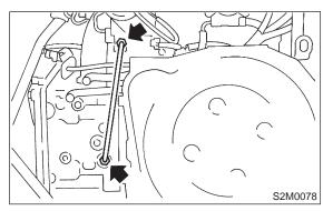
21) Remove engine harness bracket from transmission housing, and disconnect engine harness connectors from bulkhead harness connectors.
