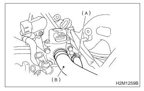
13) Connect engine coolant hose to throttle body.
