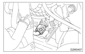
7) Remove bolts which install idle air control solenoid valve, and move it. <Ref. to 2-7 [W13A0].>
