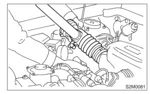
6) Disconnect connector from engine coolant temperature sensor.
