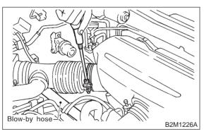
4) Disconnect emission hoses from air intake duct.
