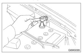
2) Disconnect connector from camshaft position sensor.
