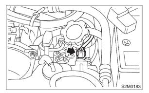
3) Remove camshaft position sensor from camshaft support LH.
