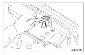
2) Disconnect connector from front oxygen sensor.
