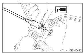
2) Install front oxygen sensor.
