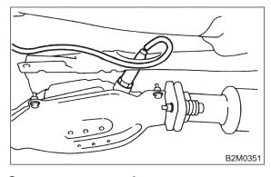
3) Connect connector of rear oxygen sensor.
