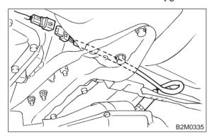
4) Apply SUBARU CRC or its equivalent to threaded portion of rear oxygen sensor, and leave it for one minute or more.
