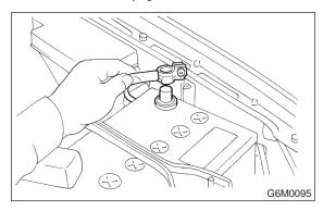
2) Disconnect connector from throttle position sensor.
