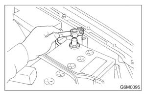
2) Disconnect connector from rear oxygen sensor.
