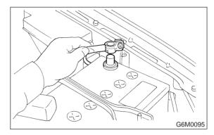
2) Loosen clamp which connects air intake duct to mass air flow sensor.
