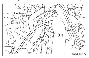
8) Disconnect air by-pass hose from idle air control solenoid valve.
