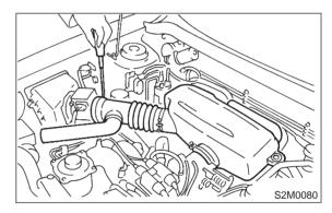
3) Loosen clamp which connects air intake chamber to throttle body.
