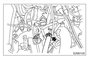
9) Remove bolts which install idle air control solenoid valve to throttle body.
