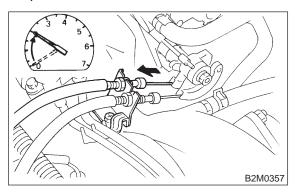
3) Disconnect air by-pass hose from air intake duct.
