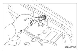
3) Disconnect connector from fuel injector.
