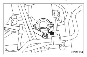
4) Remove fuel injector from fuel pipe assembly.
