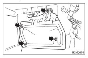
5) Remove vinyl cover and nuts which attach ECM to bracket.
