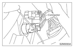
3) Remove fuel pump relay from mounting bracket.
