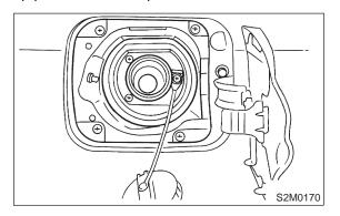
5) Connect evaporation hoses to pipes.
