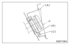
4) Insert fuel filler hose (A) approximately 25 to 30 mm (0.98 to 1.18 in) over the lower end of fuel filler pipe and tighten clamp.
