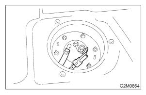
18) Connect connector to fuel pump relay.
