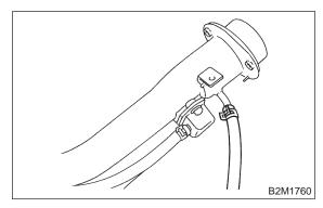
4) Connect evaporation hose to evaporation pipe.
