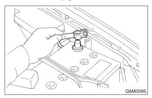
4) Drain fuel from fuel tank. <Ref. to 2-2 [W9C0].>
