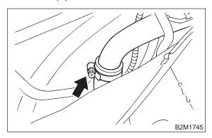
18) Remove fuel filler pipe to under side of vehicle.
