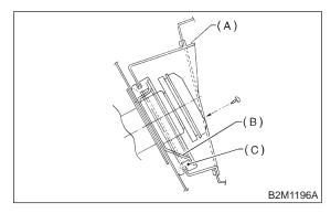
3) Align holes in fuel filler pipe neck and set cup (B), and tighten screws.
