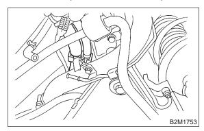
9) Connect evaporation hose to joint pipe.
