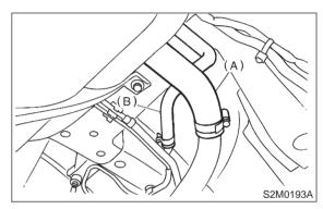
10) Remove fuel filler pipe to under side of the vehicle.
