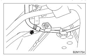
17) Loosen clamp, and disconnect fuel filler hose from fuel filler pipe.
