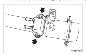
2) Connect evaporation hoses to shut valve.
