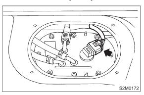
17) Install fuel sub meter unit, and connect connector and jet pump hose. <Ref. to 2-8 [W8A0].>
