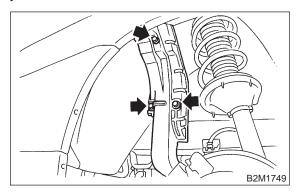
12) While releasing the under side of protector cover from hook, remove it.
