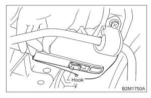
13) Disconnect evaporation hoses from pipes.
