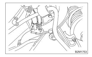
16) Disconnect evaporation hose from joint pipe.
