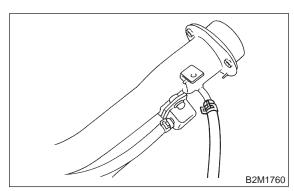
4) Disconnect evaporation hoses from shut valve.
