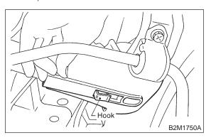
12) Tighten bolts which install protector cover on body.
