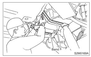
2) Move clip, and disconnect evaporation hose from fuel cut valve.
