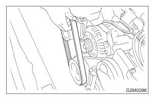
(4) Remove generator lock bolt.
