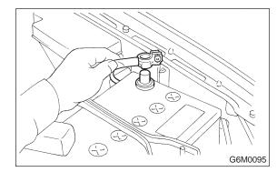
7) Start the engine, and measure oil pressure.
