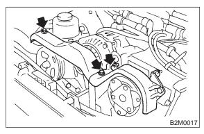
(3) Loosen lock bolt and slider bolt, and remove front side V-belt.
