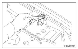
2) Remove generator from bracket.(1) Disconnect connector and terminal from
