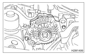
3) Disconnect connector from oil pressure switch.
