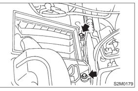
(8) Disconnect spark plug cords from spark plugs (#1 and #3 cylinders).
