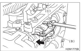
(7) Insert tweezers into the notch of the valve lifter, and take the shim out.
