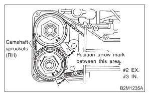
(2) Set arrow mark on camshaft sprocket to position shown in figure, and check #2 cylinder intake valve and #4 cylinder exhaust valve clearances.
