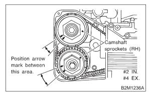
(3) Set arrow mark on camshaft sprocket to position shown in figure, and measure #1 cylinder exhaust valve and #4 cylinder intake valve clearances.
