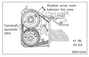
10) Measure #1 cylinder intake valve and #3 cylinder exhaust valve clearances by using thickness gauge.
