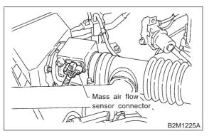
(2) Loosen clamp which connects air intake duct to air intake chamber.
