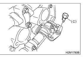
(6) Rotate REPLACER No. 3 until REPLACER No. 2 pushes away valve lifter.
