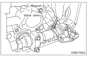
4) Measure thickness of shim with micrometer.
