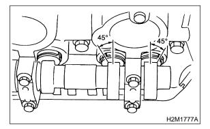
(3) Set REPLACER No. 1 (A) to exhaust camshaft.
