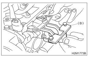
(5) Set REPLACER No. 3 (C) to hole of REPLACER No. 1.
