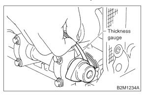
11) If necessary, adjust the valve clearance. <Ref. to 2-2 [W7B0].>
