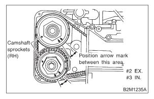
(2) Set arrow mark on camshaft sprocket to position shown in figure, and measure #2 cylinder intake valve and #4 cylinder exhaust valve clearances.
