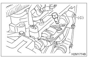
(6) Rotate REPLACER No. 3 (C) until REPLACER No. 2 (B) pushes away valve lifter.
